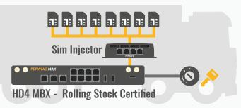
The HD4 MBX comes with multiple features to make it ideal for on-the-go deployments. Ignition Sensing gives it the ability to turn on and off depending on whether the vehicle has started. Upon vehicle shutdown, the MBX can also shut down after a user-defined interval, saving the battery from excessive drain.
